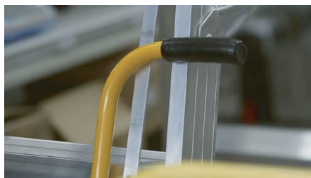
One control raises the unit to the mobile position and provides easy positive steering
